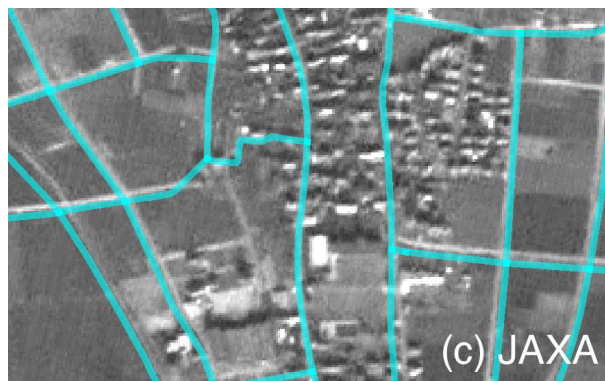
Fig. 2 Typical difference of ALOS/PRISM imagery and NTIS road features (light blue).
