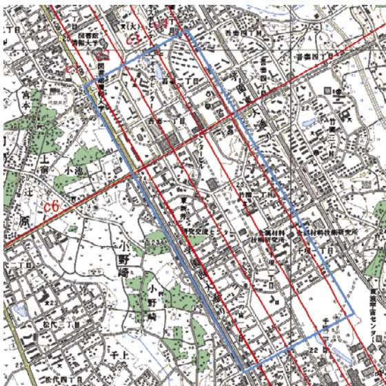
Fig. 6 The target area and the flight tracks. Red number indicates course no. Course 5 is only used for integrity check.
