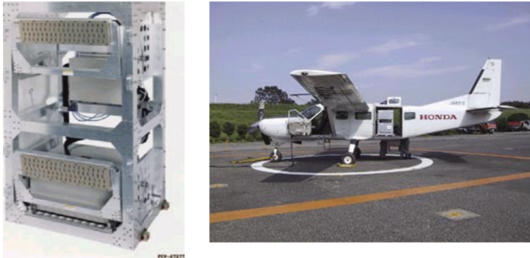
Photo 1 Assembled airborne SAR equipment used for the repeated measurements over the Asama volcano on September 16, October 22 and December 15, 2004 (left). The aircraft (Cessna 208) with onboard SAR instruments mounted (right).
