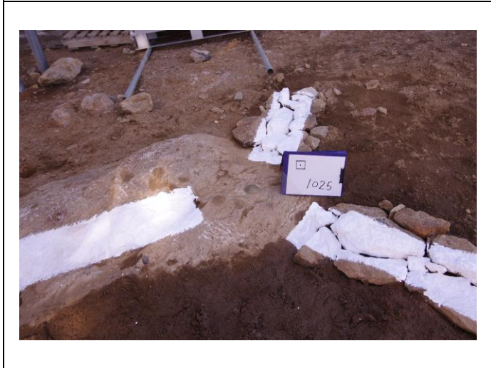
対空標識写真 Airphoto Signal Photograph
