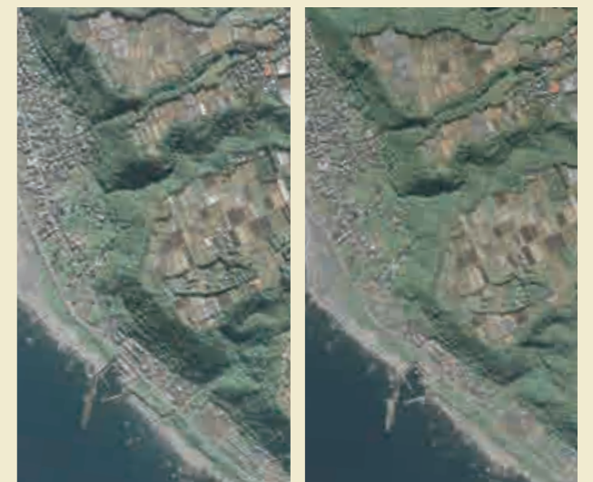
By setting up a partition between photos, and viewing the left photo with the left eye and the right photo with the right eye, we can get a 3-dimensional view of the undulations of the terrain.
