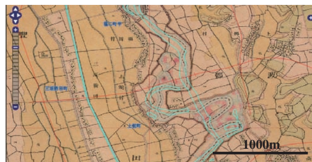
Fig.19a Overlay of “Jinsoku-sokuzu” published by the Imperial Japanese Army in the early Meiji period and Fundamental Geospatial Data published by GSI on the present day Yoshino area, Joso City (by Historical Agriculture Environment Inspection System of the National Institute for Agro-Environmental Science). The light blue colored areas are water areas and the dark blue colored areas are wetlands in the early Meiji Era, and blue solid lines represent present water boundaries.
