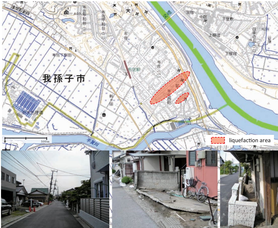
Fig.12 Liquefaction damage in the Fusa area, Abiko City (base map by GSI Maps), and ground photos taken in a field survey on 3rd June, 2011
