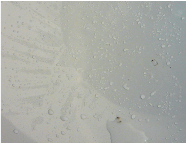
Fig. 8 The inside of the radome of 06S061 when the large errors in the vertical displacements time series are observed. Many water droplets are seen on the surface.
